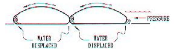
The AquaDam® is able to offer a stable wall by containing two water columns in a single outer tube. The contained water columns are unable to assume their natural position and form a vertical wall in the middle as they press against each other. The pressure inside the tubes applies a substantial force to both sides of this vertical wall.
