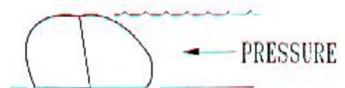
In order to move or tip a filled AquaDam®, the maximum recommended working depth would have to be exceeded. Too much water pressure against the side may cause the entire AquaDam® to slide or tip sideways, depending on the nature of the surface and friction factor it is placed on. It would be technically impossible for one tube to roll completely over another in a filled AquaDam®.
