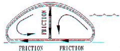
As water pressure builds on one side of the AquaDam®, the pressure displaces the water in the inner tubes. However, because the inner tubes are unable to move, the AquaDam® assumes a position of equilibrium and behaves as a solid dam.
