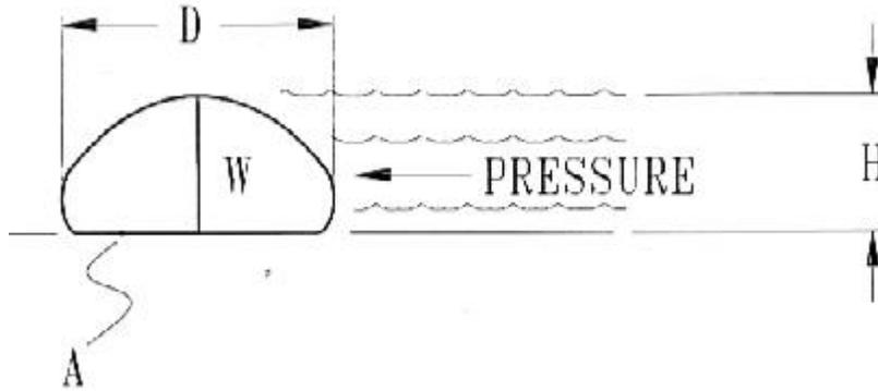
In order for an AquaDam® to move as a result of the pressure exerted on one side, it must slide across the surface on which it rests. In order to tip, the water pressure must lift the first inner tube up and over the second. The following calculations show the AquaDams® resistance to tipping:
