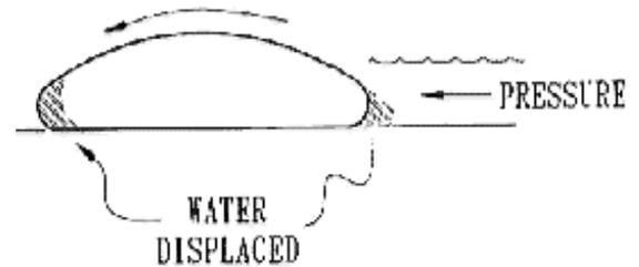
Two water-filled tubes or columns placed side-by-side will assume their natural shapes. If pressure is applied to one side, the water is displaced in the first tube and causes it to roll. As the first tube rolls, it pushes on the second tube moving the water from one side to the other and the two tubes roll together.
