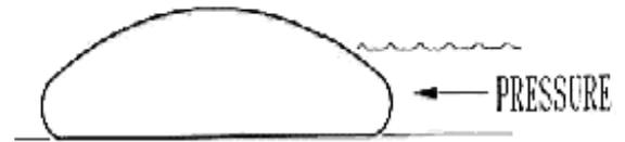
As a result of the building pressure, the water is pushed from one side of the tube to the other side where the pressure remains low. As the water continues to move from one side to the other, the tube begins to roll.
