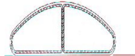
As water pressure begins to build on one side of the AquaDam®, the inner tube naturally tries to roll. However, the friction between the vertical walls and between the inner and outer tubes opposes the rolling tendency and the structure remains fixed.
